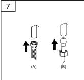
Connect water supply lines. (A) Use 1/2" IPS faucet supply lines or (B) use coupling nuts (not supplied) with ball-nose risers (not included). Turn water supply or shut-off valve back on and check for leaks. If leaks occur, gently tighten the faucet connections.
